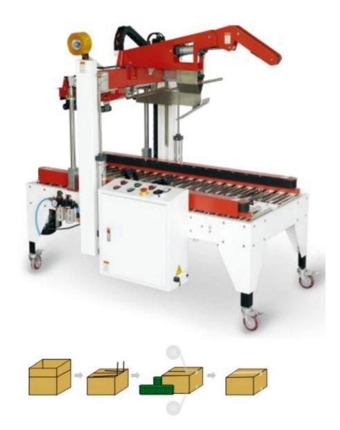
Automatic cover carton sealer suitable for the use of various specifications of carton at the same time, automatic size adjustment when changing specifications, using belt drive, can pack 900 cases/hour
