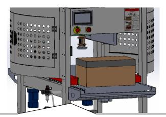
Rotate this shaft with a handle to make the conveyor belt close to the packing case (Note: It is necessary to master the friction between the conveyor belt and the packing box, too much friction will cause deformation of the packing box, too small carton may slip and can not be sent out), Rotate the left and right conveyor belts clockwise to close (and vice versa).
