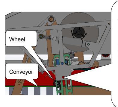
The two M12 bolts are rotated counterclockwise for two turns with a hexagon plate to loosen the sealing head, and the sealing head is moved to move the pressure belt rubber wheel to about 10mm beyond the conveying line. Then the two M12 bolts are twisted clockwise with a hexagon plate. (Note Ensure that the device is at the origin before adjustment)
